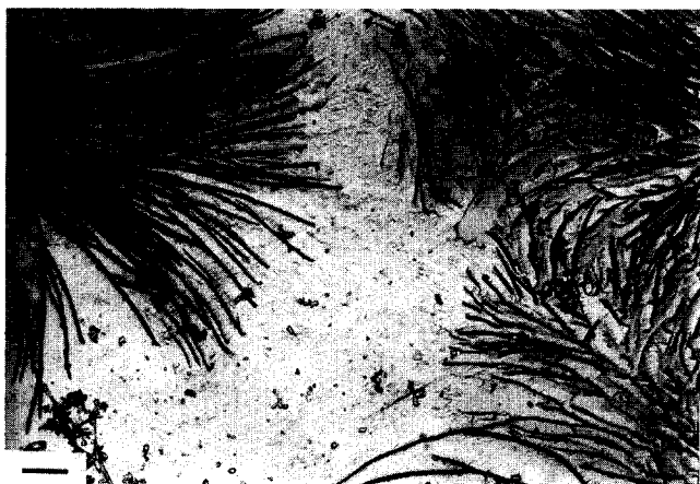
Figure 5 TEM micrograph of a replica of the fraction EBb(2.1), after isothermal crystallization at 120°C for 60 h. No further crystallization is observed in samples that have been held isothermally at 120°C for 1 week; all possible crystallization has taken place after 60 h. The polymer which has crystallized isothermally is found in large spherical domains; this is clear evidence of phase separation in the melt from which the crystallization took place 2,6 . The scale bar represents 1 μm
